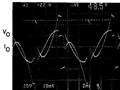
FIGURE 9. Reaching the SOA Power Limit, f = 100\text{ Hz} , SPiKe Enabled
